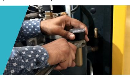
Refill oil up to the middle of the sight glass or as recommended by the air compressor manufacturer
