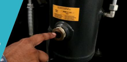
**Example :** In this case (and in video from MVS) the sight glass is on the air receiver, marked by '5' in the diagram below
