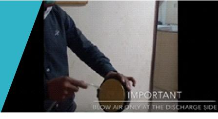
Continue blowing jet of air on side of filter also pointing downwards.
