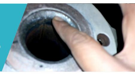
If CMS level is below the top flange of PSA tower, fill CMS in the tower until the CMS level has reached top flange of the PSA tower
