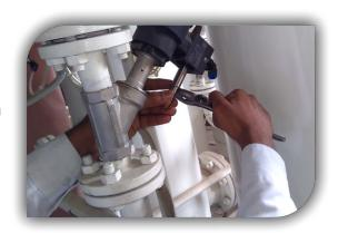
Remove plunger and clean carefully with clean and dry compressed air.
