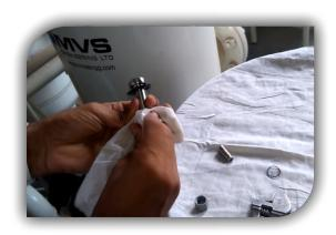
Reassemble plunger carefully inside solenoid valve
