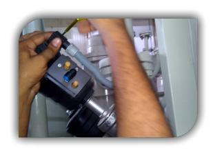
Open solenoid valve by using Allen key
