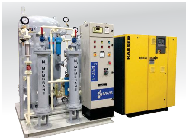
I-ZEN Industrial Unit with integrated compressor. Nitrogen membranes - 50 Nm 3 /hr Nitrogen flow
