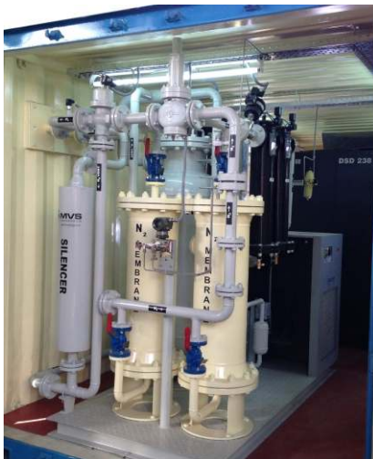
C-ZEN Containerized Units with integrated compressor. 300 Nm 3 /hr Nitrogen flow for Petrochemical Tanks and Oil Field application
